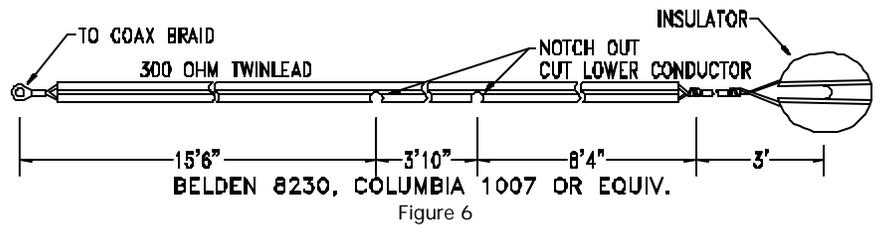
steel wire to support the weight of the radial. Four such radials will be the practical equivalent of the system shown in figure four for operation on 40 through 10 meters.
