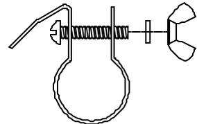
NOTE: The outer tab of this clamp may be bent back slightly to provide clearance for the bolt, bending it back into place after assembly.
