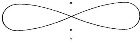
When excited "out of phase" these same verticals can be made to give an "end fire" or bi-directional pattern in the opposite direction through the plane of the verticals. This then nulls out signals in the opposite directions. More gain is exhibited by the broadside pattern over the "end fire" arrangement, but the "end fire" arrangement offers a wider frontal pattern.
